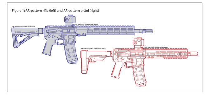
And yet, both AR-pattern rifles and AR-pattern pistols have a similar construction, using a splitframe that separates the firearm into an upper and a lower (Figure 2).
